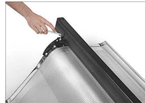
Step 2: Fasten the beam with allen keys
