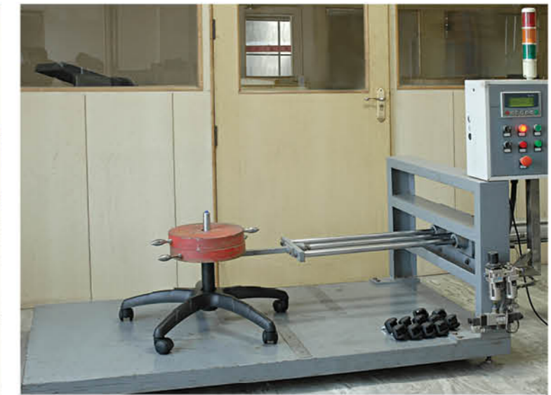
Castor Testing Machine
