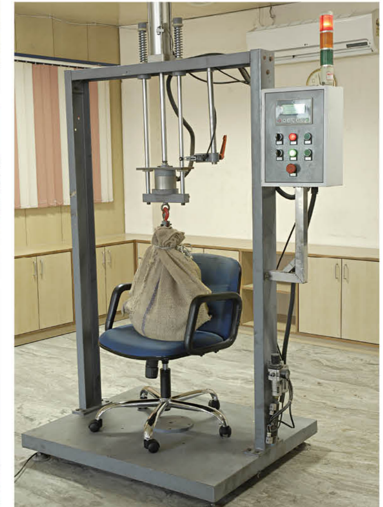
Impact Testing Machine
